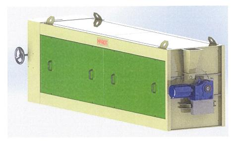
The MAROT indented cylinder separates grains according to length by size of the indentations in the shell. These shells are easily changed, allowing the machine to be altered to suit different lengths of grains.
